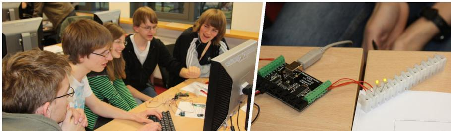
Figure 1: Pupils controlling an LED using Squeak and the Phidget InterfaceKit
